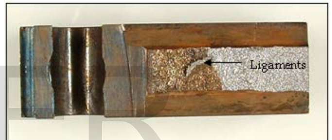
Fig.1.4: Ligaments observed in the crack wake after testing. Specimen heat treated for 100h tested at K_{applied} = 76.5 \text{ MPa}\sqrt{\text{m}} and potential of -1100mV/SCE.
